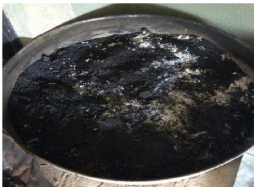
Plate 3.2 Rice husk burnt to ash by controlled burning.
