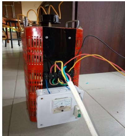
Fig 6: The Completed Variac showing external connections to the components
