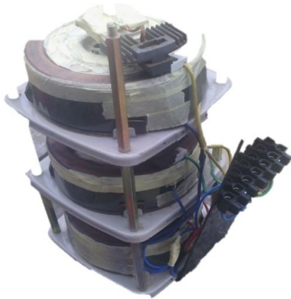
Fig 5: The Variac showing the individual cores stacked upright.
