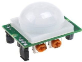
Fig. 3: The PIR motion sensor
