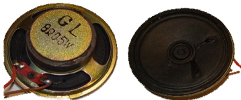
Fig. 8: 8 Ω, 0.5 W loudspeaker
